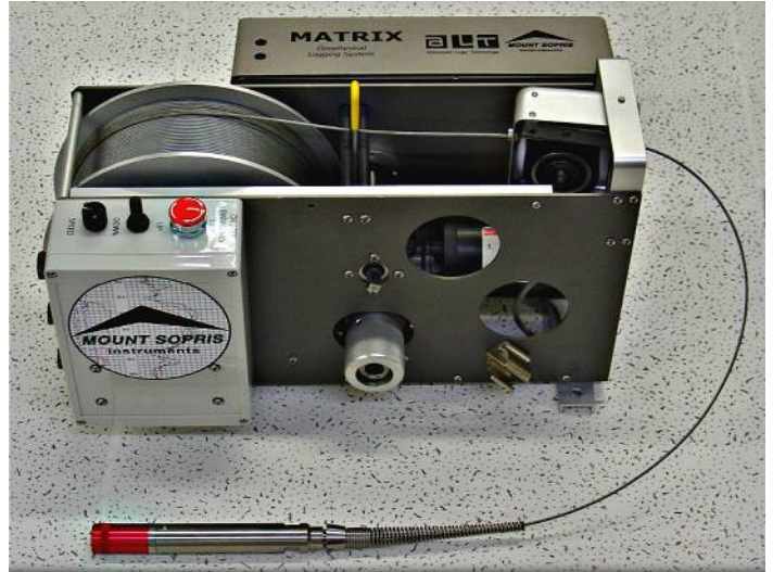
Matrix with portable winch (The winch length of the picture is 300 meter)
